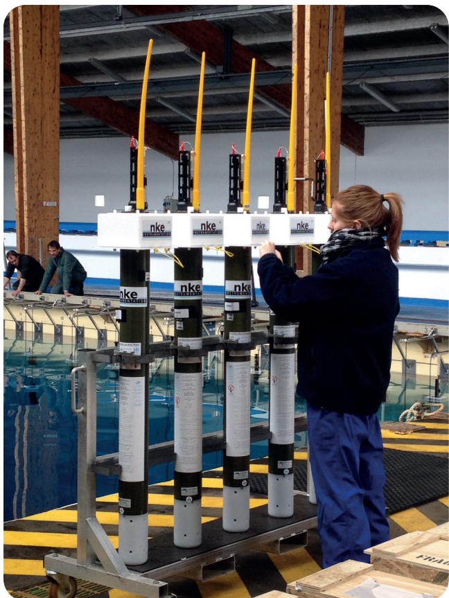
Argo floats ready to be tested at the IFREMER facility. © Olivier Dugornay/IFREMER
