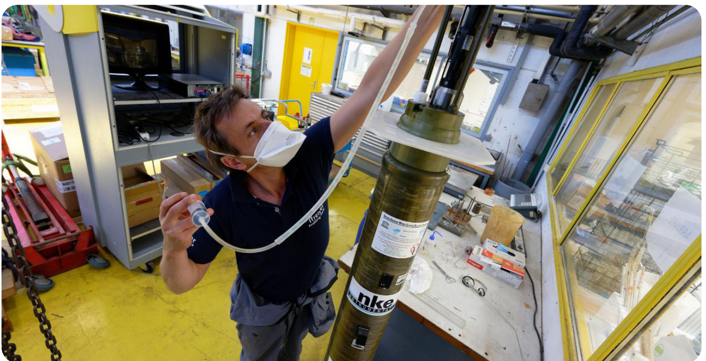
A Deep Argo float tested at the IFREMER facility. © Olivier Dugornay/IFREMER
