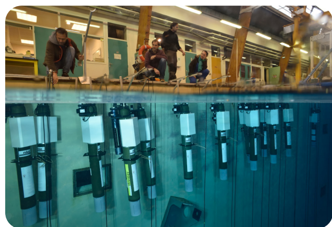
Biogeochemical floats tested at the IFREMER facility. © Olivier Dugornay/IFREMER
