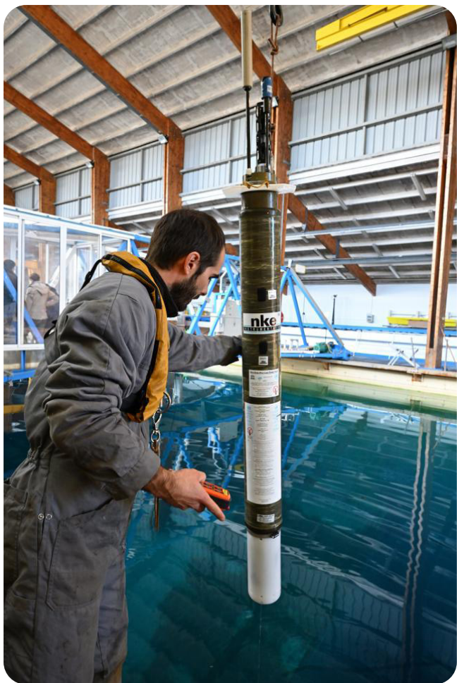
A Deep float tested at the IFEMER facility by Romain Cancouët who is in charge of all operational tasks at Euro-Argo ERIC. © Stéphane Lesbats/ IFREMER
