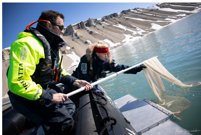
Scientists use manta trawl net to sample microplastics during GOOD-IMDOS research campaign in the Arctic, June 2023. Photo credit: Xavier Boymond
