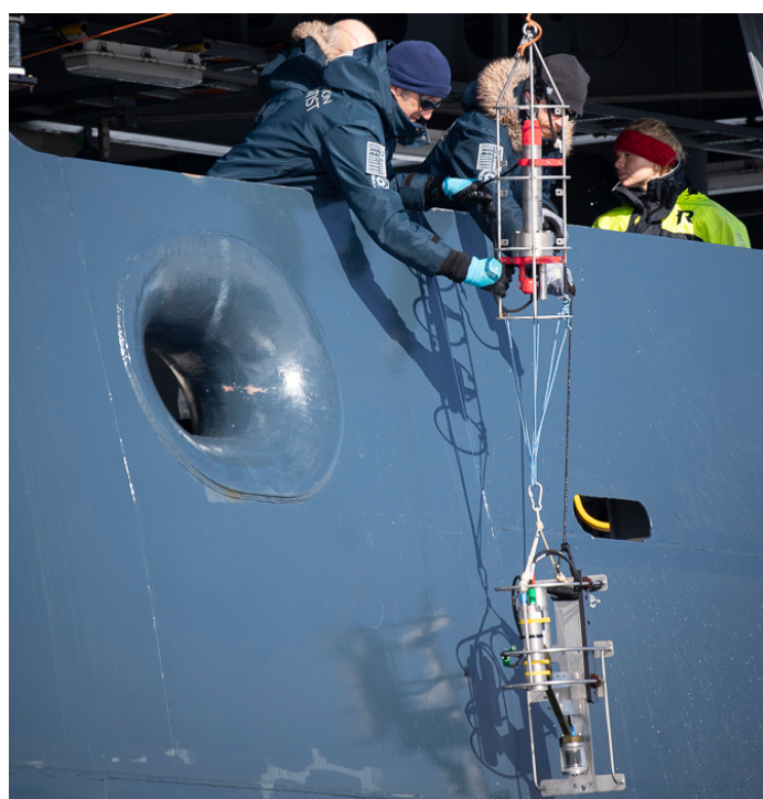
Boxhammer (right) and fellow scientist descending the Conductivity Temperature Depth (CTD) device (top instrument) and Underwater Vision Profiler (UVP) (bottom instrument) during Arctic science campaign in June 2023. Photo credit: Xavier Boymond
